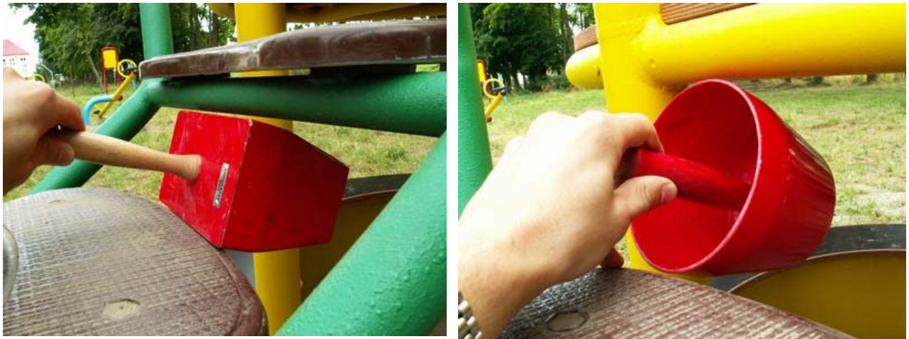
Figure 3. Head and neck entrapment. Step 1: Checking the opening with two smaller probes. If the torso (left photo) and small head probe (right photo) can pass through the opening the large head probe shall also pass through the opening (shown on figure 4).
