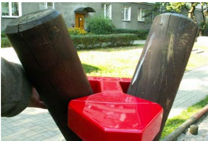
Typical places of jamming: at joints of two diagonal rungs (the picture was taken during examination of possibility of head jam) and at the end of steps.
