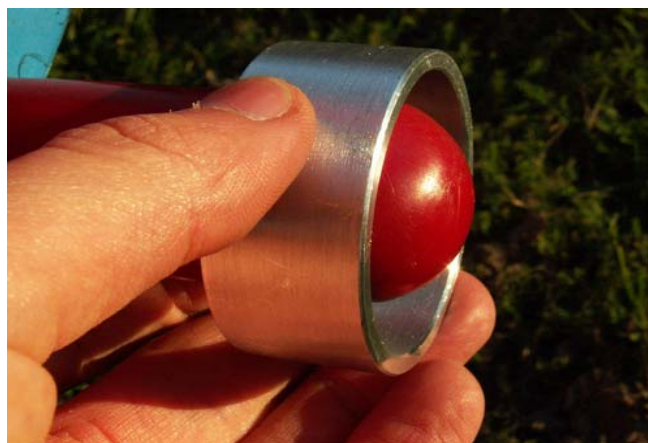
Figure 11: Testing of the hazard of eye injury. We carry out the test through setting the gauge over the end of the hand support or footrest and afterwards applying the gauge only along the centre line of the hand support or footrest.
