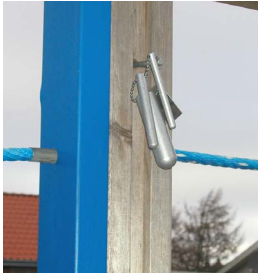
Figure 10. The finger rods are used for checking for finger traps.
