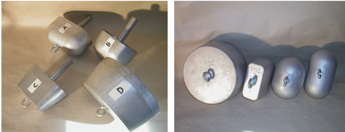
Figure 2. The two test probes A and B that are required to test for head and neck entrapment according to German legislation.
