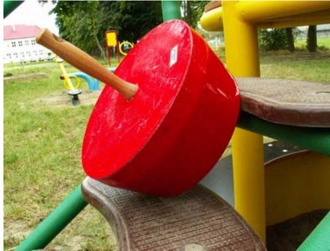
Figure 4. Head and neck entrapment. Step 2: Checking the opening with big probe. As the large head probe cannot pass (as shown on photo) this equipment possesses a risk of head entrapment.
